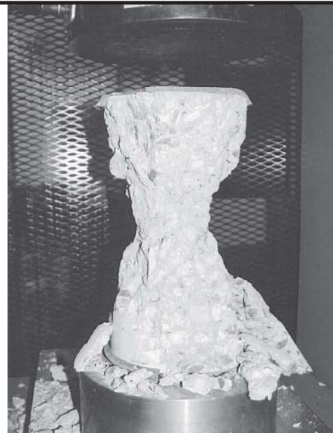
Fractured Test Specimen at Failure
